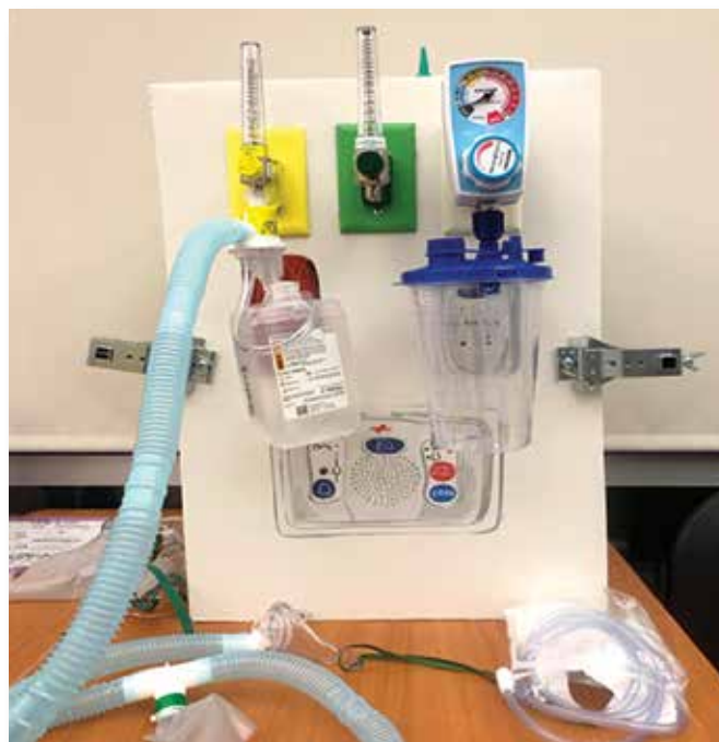
Figure 2: Closeup of the oxygen and air 50 psi interface ports.
